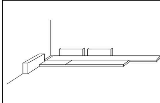
9. **Laying out the floor...** Be sure to work from multiple boxes simultaneously as you install the flooring to ensure variation and good blending of the boards throughout the entire installation. ***Impressions warranty does not cover materials with visible defects once they are installed. Installation is acceptance of product.***
