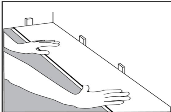
8. **Expansion Space...** Maintain proper expansion space at all side and end walls, and at all vertical obstructions. The expansion space is generally equal to the thickness of the flooring. Maintain 1/2" expansion space for Impressions 1/2" engineered hardwood flooring. The use of spacers may be helpful in maintain a straight working line.
